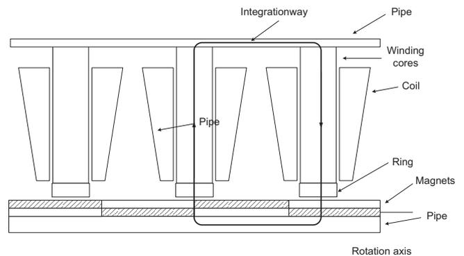
Fig. 1. Sectional drawing of the linear machine.
