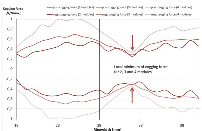
Fig. 12. Simulation results of the cogging forces by variation the ring width
