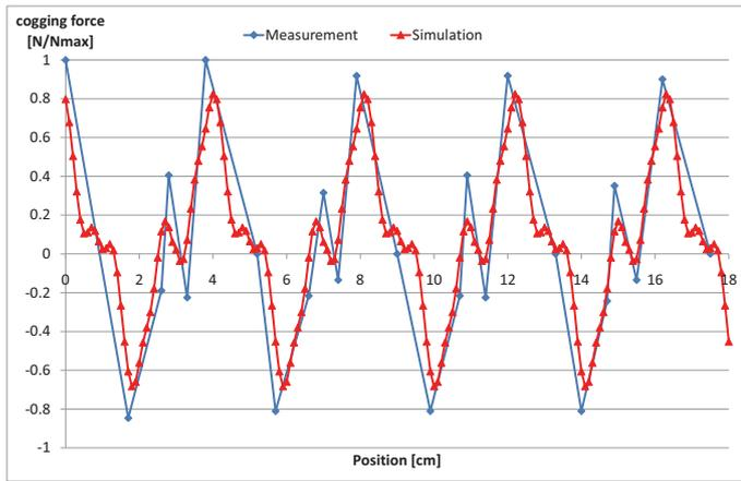
Fig. 8. Cogging forces of the constructed linear drive in comparison to the simulation
