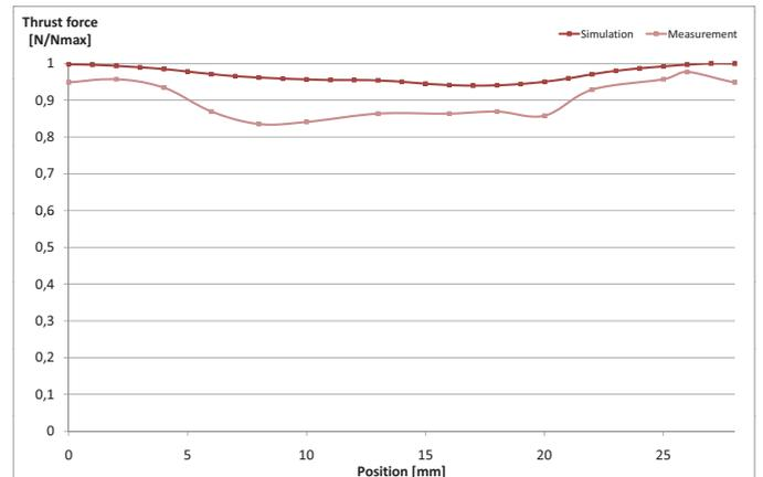
Fig. 7. Active force of the constructed linear drive in comparison to the simulation
