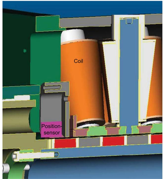
Fig. 3. Placing of the internal positioning sensor.
