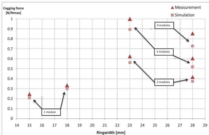
Fig. 9. Maximum cogging forces of all constructed versions of the linear drive in comparison to the simulation
