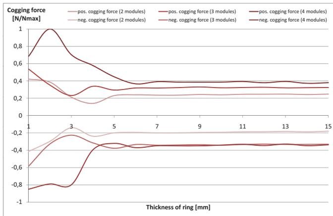
Fig. 11. Simulation results of the cogging forces by variation the ring thickness
