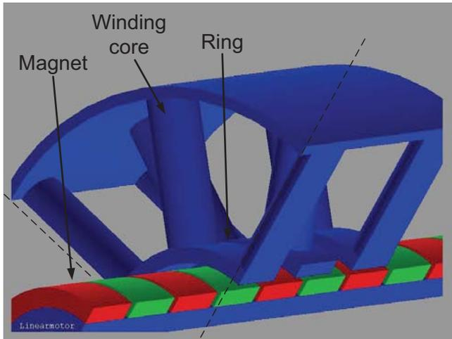
Fig. 2. Configuration of the shifted winding cores.
