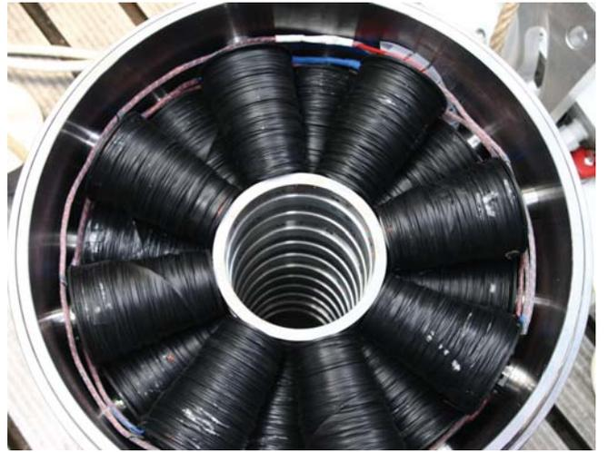
Fig. 6. Stars with discrete wound conical coils
